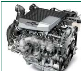
Mazda's Direct Injection Spark Ignition (DISI), developed in 2005, injects petrol directly into the combustion chamber, whereas traditional systems mix air and petrol prior to injection. Combined with the DISI TURBO system, the engine provides sharp acceleration, high torque at low and medium engine speed ranges, and also high fuel efficiency and clean exhaust emissions.
