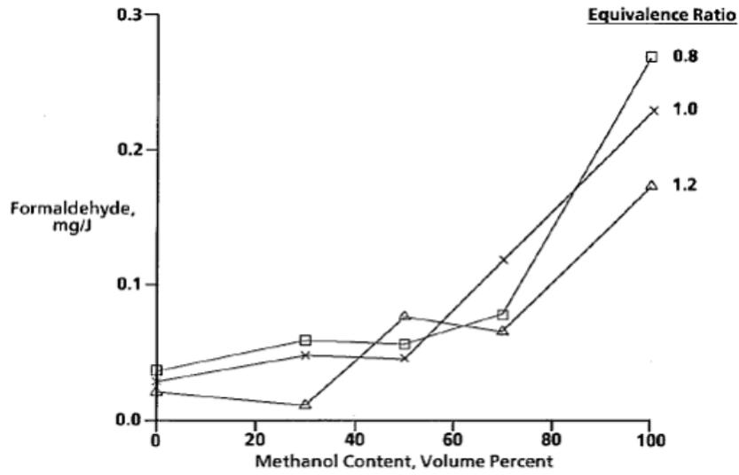
**Figure 23.** The Effect of Methanol Addition on Formaldehyde Emissions
